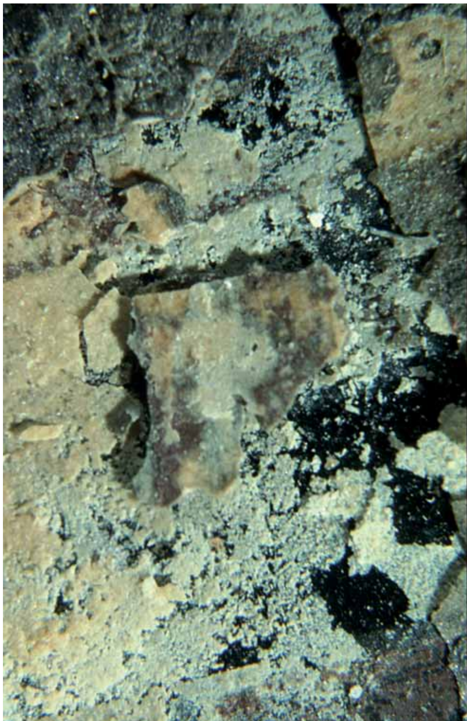
Fig. 3 - Example of chemical weathering of the glass due to the reaction between pollutants and water on an ancient stained glass window in Sainte Chapelle (Paris) (from Bernardi 2008).
